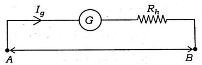
where G is the galvanometer,  $I_g$  is the current passing through the galvanometer,  $R_g$  is the galvanometer resistance,  $R_h$  is the high resistance.
